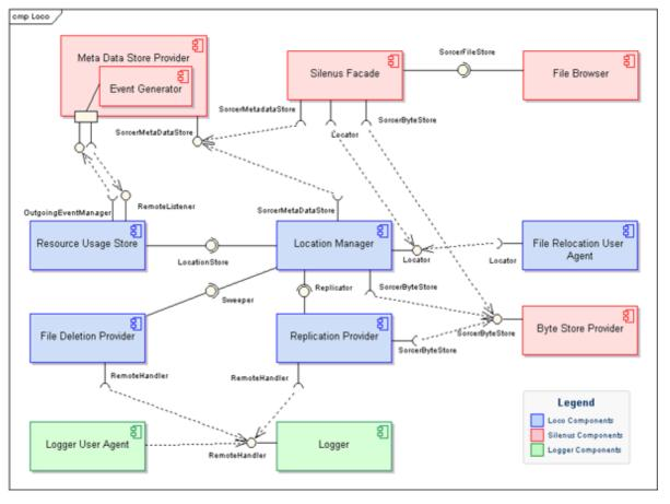
Figure 2 LOCO architecture (UML component diagram)
