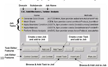
objects on the fly. The Job Editor features also enable the specification of the Control Context and the JobContext. The ControlContext specifies the flow and method of execution of the FiperJob. The final step before a FiperJob can be executed is to define the flow of data between tasks in the job. This is done using the JobContext dialog, which can be invoked from the Job Editor features on the Job Editor Dialog in Figure 8.
