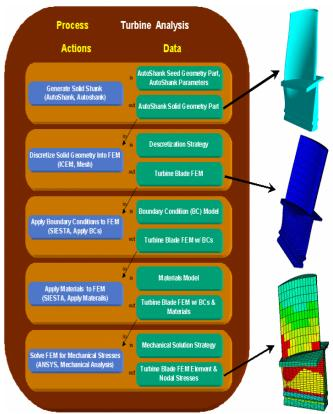
jects and act as a service requestor to submit the Figure 4. Process for the Mechanical Analysis of a Turbine Blade
