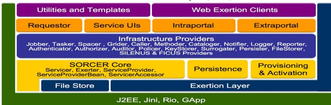
Figure 1. The SORCER layered functional architecture.
