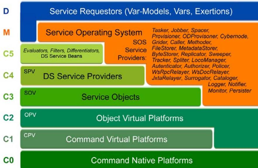
Figure 3: The SORCER layered architecture, where C0-C5 (carrier)—the metaprocessor with its service cloud at C4 and C3, platform cloud at C2 and C1, M (management)—SORCER operating system, D (domain)—service requestors; where PV and OV stands for provider and object virtualization respectively with the prefix S for service, O for object, and C for command.
