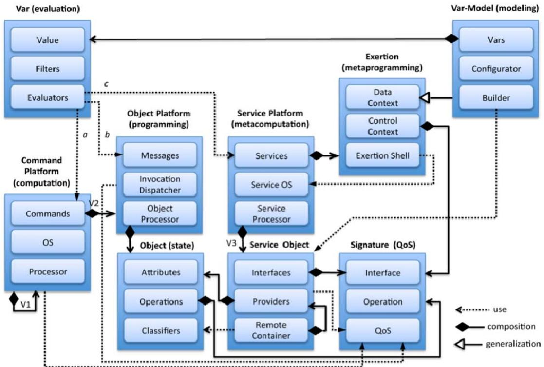
Figure 2: The SORCER metamodeling architecture: evaluation, modeling, metaprogramming, metacomputation, programming, and computation. Each platform is shown as the DMC triplet (domain, management, carrier). The service platform manages the service providers (service cloud) that are autonomically provisioned by service objects on virtualized object/command platforms.
