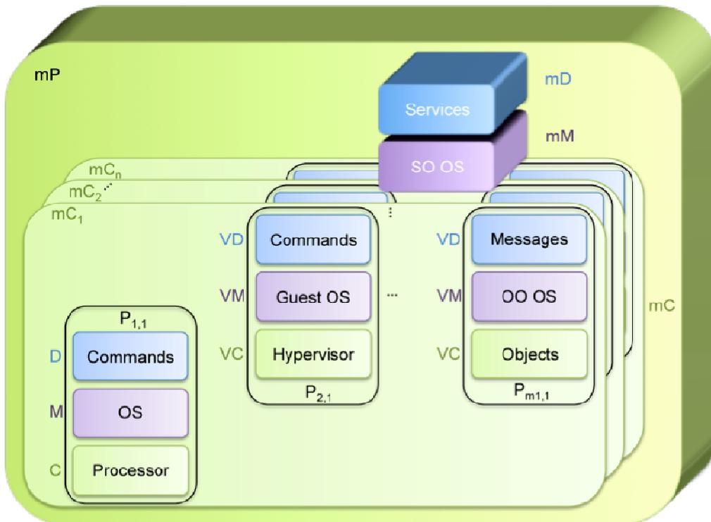
Figure 1: Software cannot operate without a platform or be platform independent. The cloud platform (mP: mD/mM/mC) with its meta-domain (mD), meta-management (mM), and meta-carrier (mC) is composed of n distributed platform clouds mC<sub>i</sub>, i = 1, 2, ..., n.
