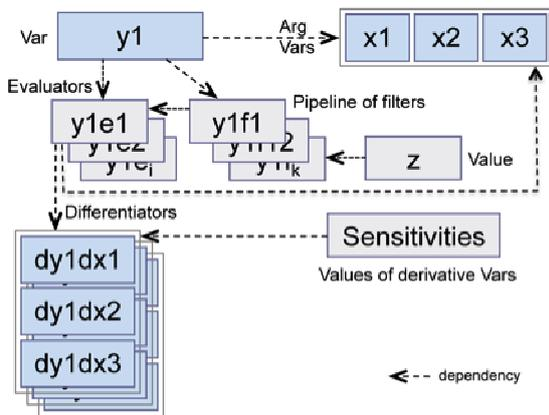
Figure 4: The var structure: value/filter/evaluator. Vars are indicated in blue color. The basic var  $y1, z=y1(x1, x2, x3)$ , depends on its argument vars and derivative vars.
